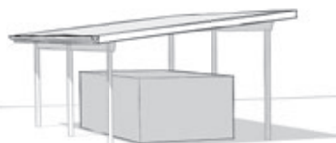
FREE ROOF BLOCKAGE > 75%
