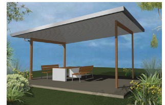
FREE ROOF BLOCKAGE < 75%
