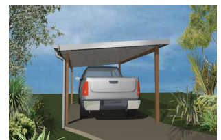
FREE ROOF BLOCKAGE > 75%
